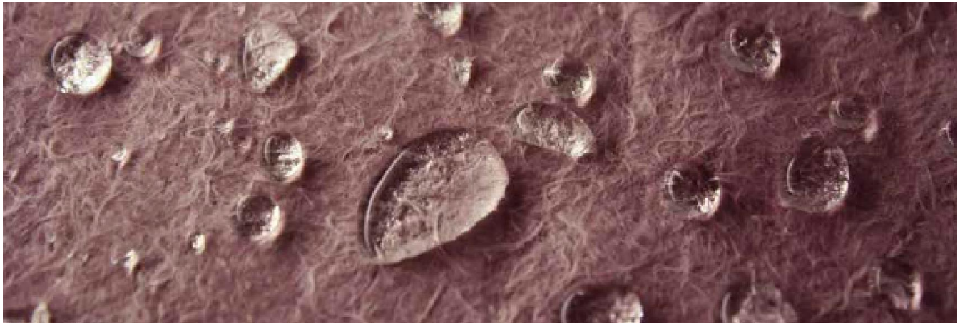
Picture of hydrophobic Pyrogel insulation used in SolaraRay panels
